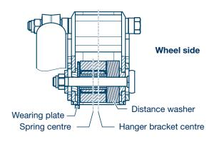
With BPW air suspension axles with adjustable aluminium hanger brackets, the head of the spring bolt is secured from rotating by means of a profiled lot in the adjusting plate.
