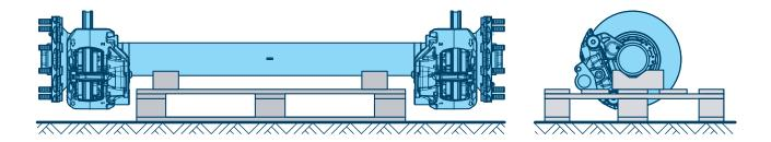
When transporting and storing the axles, a suitable rack or support should be used to avoid impacts, e.g. on the brake disk rim.
