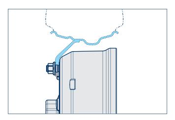
3. Use only rims which ensure sufficient clearance to the brake drum and all installed brake components.
