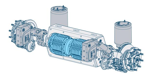
With ePower, BPW offers a trailer axle with integrated generator transmission units (GTU). These generate electricity for consumers in the trailer, e.g. for refrigeration machines, when driving downhill or decelerating the vehicle.
