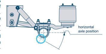
The triangle in the BPW logo is in the centre and can be used for holding a measuring tool: The maximum possible wheelbase correction per axle is  $\pm$  10 mm (see page no. 212) for tracking plates and  $\pm$  5 mm (see page no. 211) for adjustable hanger brackets.
