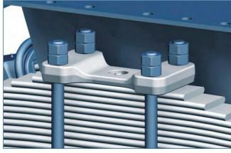
**Leaf spring clamping** by forged spring plates with high strength
