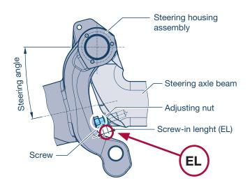
BPW self-steering axles are designed for steering angles of up to 20°. A special axle beam shape is optionally available that allows a steering angle of up to 27° (only for square 120 solid).
