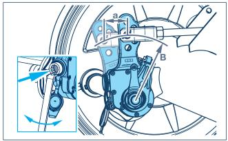
12. Set the idle stroke "a" to 10 - 15 % of the connected brake lever length "B" by turning the adjusting hexagon (again, press down the coupling sleeve with a ring wrench). Example: brake lever length 150 mm => empty stroke 15 - 22 mm.
