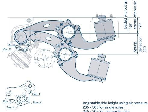
Pinning position for the two-sided axle lift
