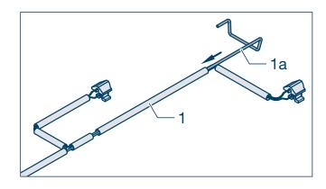
1. Pre-mount the retention clip (1a) in the protective sleeve of the cable (1) as shown.
