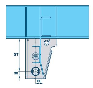
Example of a general bracing proposal for in longitudinal direction torsionally stiff vehicle frames (tankers, silos, box-body trailers) and for especially tough use.
