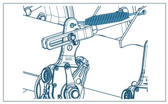
9. The outer return spring is no longer required on BPW brake cylinders with round-hole fork heads.
