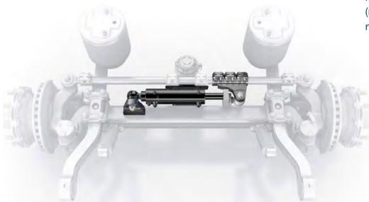
The optional electrohydraulic plug-and-play system ARC automatically ensures the correct steering angle in every reversing situation. The locking cylinder is only required in the event of a malfunction of the ARC (manual on / off switch). The switching signal comes via the EBS or the reversing light.
