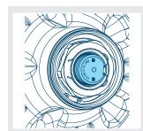
If the type plate is lost: Use the axle beam welding number on the spindle (right side).
