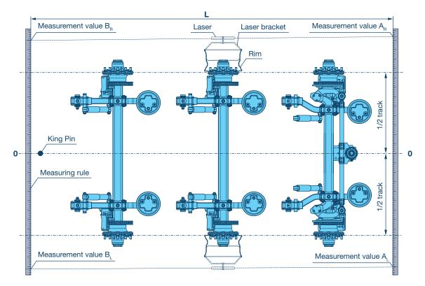
To compensate for manufacturing tolerances, an axle alignment check must be conducted and any corrections made as necessary.
