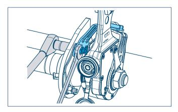
11. Secure plate with two hexagon bolts and lock nuts to inner side of supporting bearing (Tightening torque M = 28 Nm).
