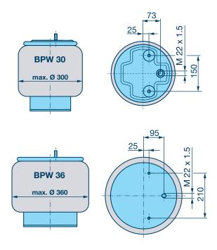
The various air bag lengths (K, Standard, -1) result in various spring deflections and lifting heights (e.g. 190 mm, 220 mm, 260 mm at axle centre). Greater spring deflections are generally more suitable for off-road use to ensure the required axle load equalization.
