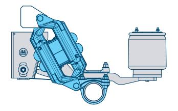
The central axle lift is located in the centre of the axle and used for lifting the centre (rear) suspension axle or if space is limited.
