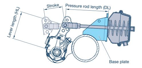
The brake cylinder mounted on the base plate transmits its force to the slack adjuster via the cylinder pressure rod by means of the fork head. The brake camshaft thus undergoes a rotary motion and spreads the brake shoes, which then rub against the brake drum.
