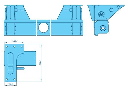
The open, narrow hanger brackets on the channel crossmember are 90 mm wide and can also be welded on to very narrow longbeam bottom flanges.
