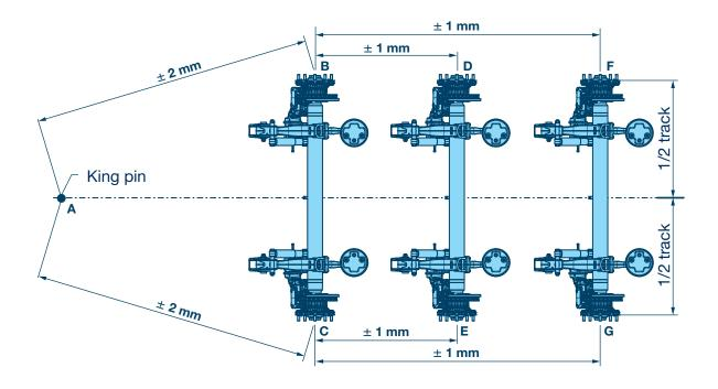
To compensate for manufacturing tolerances, an axle alignment check must be conducted and any corrections made as necessary.
