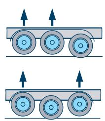
It is recommended to raise the front axle of a suspension due to the improved ground clearance (gradient of superstructure) and the longer wheel base, thus resulting in more stable driving characteristics.
