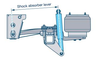
Shock absorbers located at the rear with large stroke therefore have a bigger lever but flatter characteristics curve. The increase in damping torque with rising lever is non-linear as the damper speed, and therefore forces, increase as well. Overall, the damping effect of dampers located at the rear is higher.
