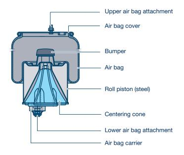
This design (Kombi-Airbag) provides unrestricted usability of vehicles with air suspension for intermodal transport.
