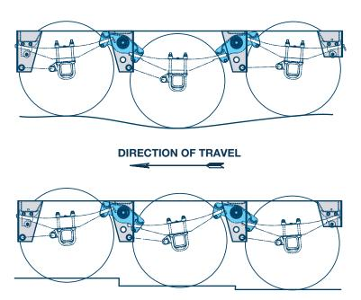
The design causes that no dynamic axle load equalisation is provided (uneven axle load distribution when braking).
