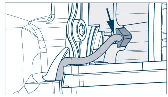
8. Clip the wear contacts into the recesses on the brake linings.
