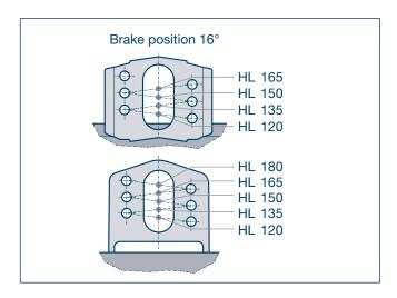
4. Mounting BPW brake cylinder on base plate
