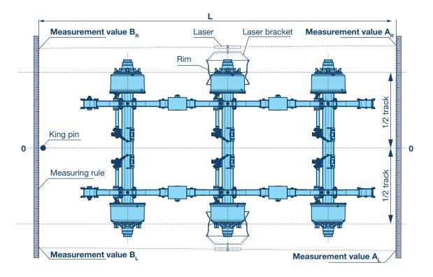
If laser measuring systems are used, care must be taken to ensure that the axle is aligned **horizontally** in order to obtain a correct measurement as otherwise the camber values will affect the result. It is assumed that the vehicle does not carry any loads.
