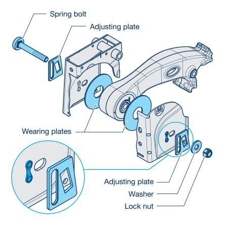
With ECO Air running gear systems, the head of the spring bolt is secured from rotating by means of a profiled lot in the adjusting plate.
