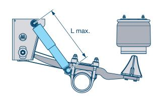
BPW shock absorbers are matched to the vehicle, overall height, installation position and applications. For air suspensions with split bags (Kombi-Airbag), the shock absorbers also act as an end stop to prevent further lowering of the axles.
