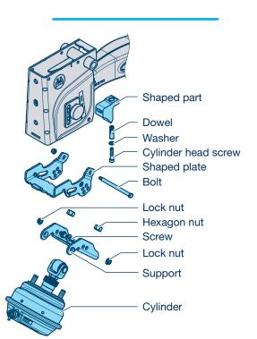
The two-sided lift is suitable for disc and drum brakes.
