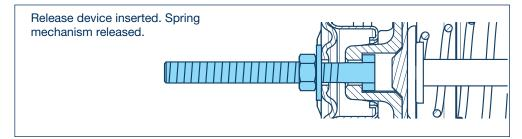
The brake cylinder release bolt must be installed in one of the two possible parking positions before vehicle is taken into operation.
