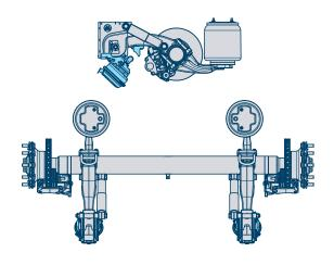
Can be used on all axles except long-stroke air For raising the front axle bags. Installation space in front of the hanger brackets and in the centre of the vehicle remains free.
