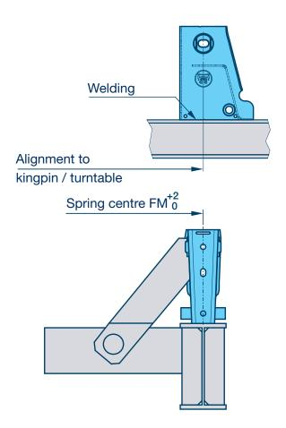
As a rule, air suspension axles are installed with the vehicle frame on its back.
