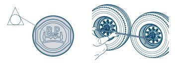
This method only takes into consideration the axle distances but not the individual track values on the axle sides. This is sufficient for axles with optimal track values. This conventional method has a higher probability of incorrect measurements than the laser method (see page no. 210). The measurement of smaller differences across greater lengths can be impacted by factors such as the elasticity in the measuring tool (manual force).
