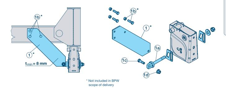
As the torsion protection of the screwed joint is created by the spring bolt flange, the bolt must always be attached to the vehicle frame through a gusset plate.
