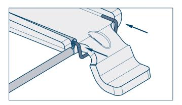
3. Push the retention clip onto the pad retainer in the direction of the arrow.
