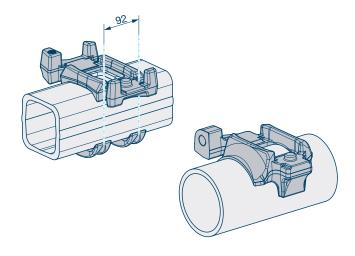
The welded Airlight II axle connection contains the spring U-bolt M 24 (SW 36).
