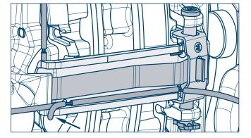
7. Mount the new pre-assembled pad retainer with brake pad wear sensing.
