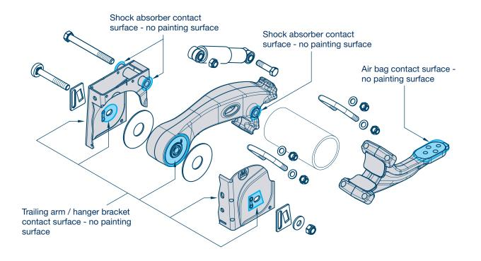
nuts, brake discs, brake lining shaft, exciter rings, ABS sensors, disc brake cylinder contact surfaces (unless already installed), all hanger bracket contact surfaces (internal and external) and the bolt-on parts of the spring bolt bearing, bolt-on parts of the shock absorbers and the air bag contact surface on the air bag carrier.
