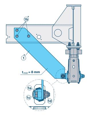
5 screws per hanger bracket, take note of the direction of installation!
