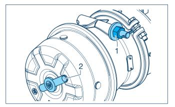
13. The mechanical release device on the spring brake cylinder must be dismantled after assembly or adjustment and inserted in the holding device (parking position) provided for this purpose.
