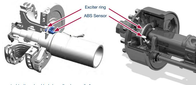
The exciter ring is connected to the wheel hub (usually clamped). An inductive ABS sensor mounted on the axle beam measures the wheel speed for the electronic braking system (EBS). This enables functions such as automatic anti-lock braking (ABV or ABS), the electronic stability program (ESP) or roll-over prevention (RSP). The spacing of the exciter ring teeth is based on the rolling circumference of the wheels.
