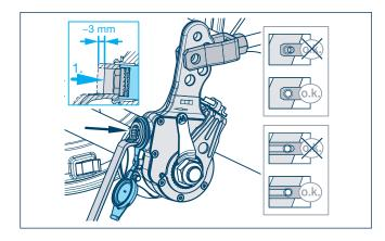
8. Remove rubber cap, press down coupling sleeve with ring wrench (width across flats 19) by approx. 3 mm (arrow) and align bolt hole in brake lever exactly with round hole or end of slotted hole in fork head by turning to the left or right. Insert and secure the bolt.
