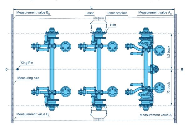
To compensate for manufacturing tolerances, an axle alignment must be conducted and any corrections made as necessary.
