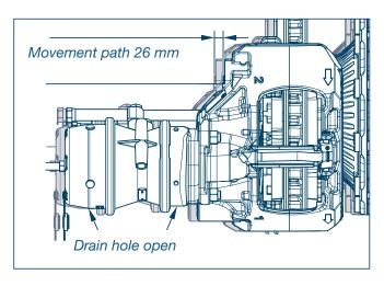
When disc brake axles are installed, ensure smooth movement of the floating calliper and all add-on pieces!
