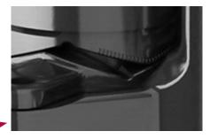
Undulated pressure disc, steered position
