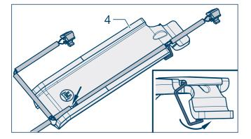
2. Insert the offset, long side of the retention clip into the bore hole in the pad retainer (2) (arrow).
