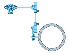
In addition to conventional air suspension valves operated by lever mechanisms, electronic air suspension modules are often found in vehicles on the market. The conventional air suspension valve is replaced with a robust ride height sensor and a multifunctional air suspension block is added.
