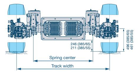
Possible track widths / spring centers for ePower: 2040 / 1300; 2095 / 1300; 2140 / 1400
