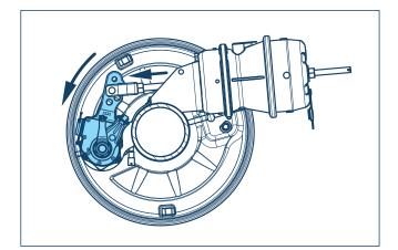
1. When braking, it is important to ensure that the rotational direction of the brake camshaft and the operating direction of the slack adjuster correspond to the rotational direction of the wheel. Otherwise, low-frequency noise may result.
