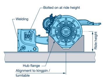
As a rule, air suspension axles are installed with the vehicle frame on its back.
