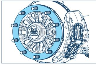
The following areas of the disc brake must be covered before any painting work:
