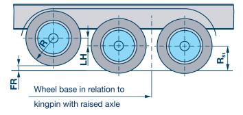
The ride height of air suspension units equipped with an axle lift device should be set at a minimum of approx. 100 mm upward travel to create sufficient ground clearance beneath the raised axle.
