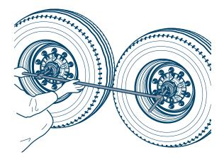
The triangle in the BPW logo is in the centre and can be used for holding a measuring tool.
