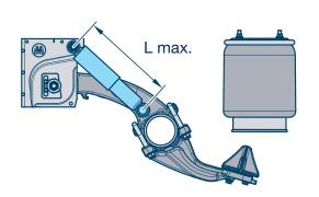
The purpose of shock absorbers is to rapidly reduce the vibrations occurring between the axle and body during driving.
