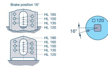
The vehicle-specific brake calculation defines the torque on the brake camshaft via the brake cylinder size and the lever length (HL). BPW offers a variable hole pattern for both the base plates and the slack adjuster to allow different lever lengths to be installed. The picture example refers to the brake position 16° for the square 120 axle beam.
