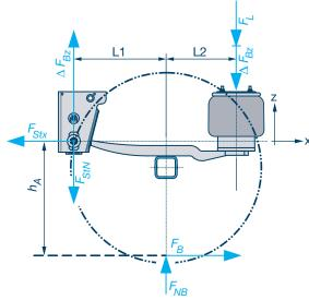
$F_{NR}$  = Wheel force on ground during braking (N)
