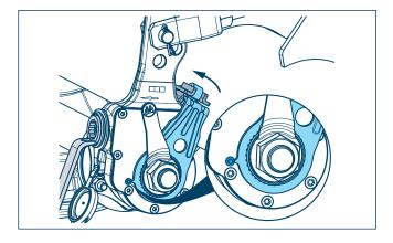
10. If the lug on the control lever still does not point to the control point, hold the coupling sleeve down and turn the control lever and shaped plate in the direction of the arrow until they reach the bumper. The lug on the control lever then points to the control point on the ECO Master (basic setting).
