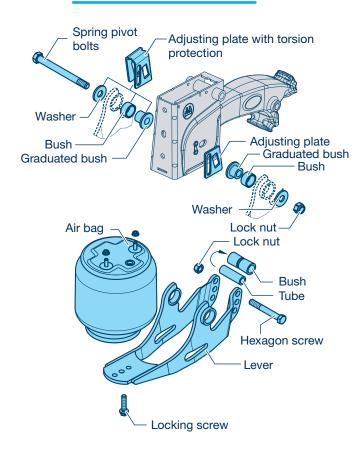
Side location is suitable for raising the front axle of the suspension unit. The lifting arm is mounted on the front hanger bracket under the trailing arm.
