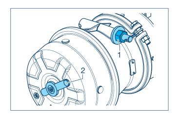
Each spring brake cylinder also contains a release device (1) for pretensioning the parking brake spring. In the delivery condition of the loose brake cylinders, the release device is clamped and thus the parking brake is released so that the cylinder can be mounted immediately. After cylinder assembly and adjustment of the slack adjuster, the release device is removed and can be parked in the lateral holding device on the cylinder.
