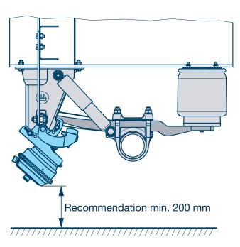
For rigid and adjustable hanger brackets, channel crossmembers and aluminium hanger brackets (not in conjunction with long-stroke air bags).
