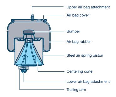
This design (Kombi-Airbag) provides unrestricted usability of vehicles with air suspension for combination traffic.
