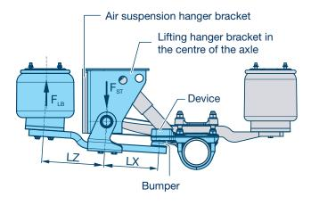
The lifting device can be arranged in the centre of the axle for lifting the central (rear) suspension axle or if space is limited.
