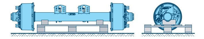
When transporting and storing the axles, a suitable rack or support should be used to avoid impacts, e.g. on the brake drum rim.
