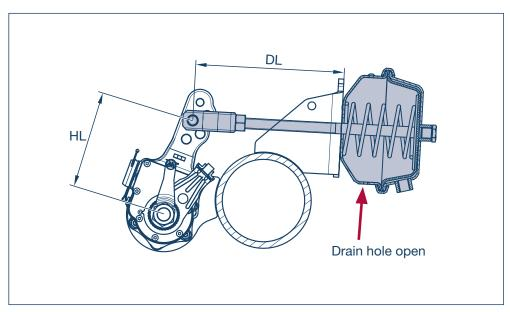
5. Set the length of the pressure rod according to the technical data of the axle.
