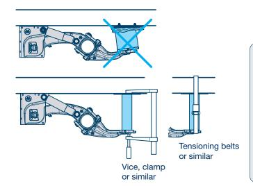
The rubber roll bag is a sensitive component and must be protected against damage during the vehicle production process, just like the
