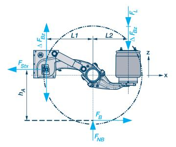
$F_{NR}$  = Wheel force on ground during braking (N)
