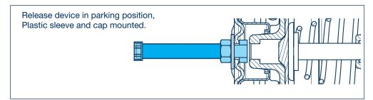
On BPW brake cylinders for disc brakes, as an alternative to the lateral holding device, it is possible to deactivate the release device by twisting. To do this, tighten the nut and fit the plastic sleeve and protective cap. The release device thus remains inserted in the longitudinal direction of the cylinder.
