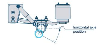
During the tracking process, the tracking values of the right and left wheel side must be averaged for each axle.
