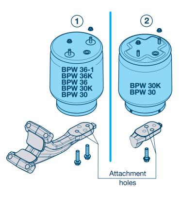
The top air bag plate is attached to the vehicle frame through the screwed joint of the 2 stud bolts (M 12).
