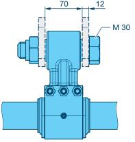
BPW also offers U-stabilizers for air suspension units with increased rolling stability requirements.
