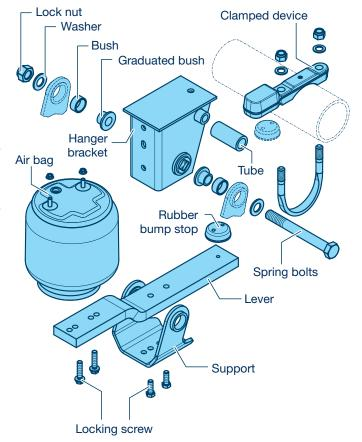
If the crossmember over the lift air bag bracket is not fitted, the torsion moment ( $F_{LB} \times L_Z$ ) of the lifting hanger bracket crossmembers must be counteracted.
